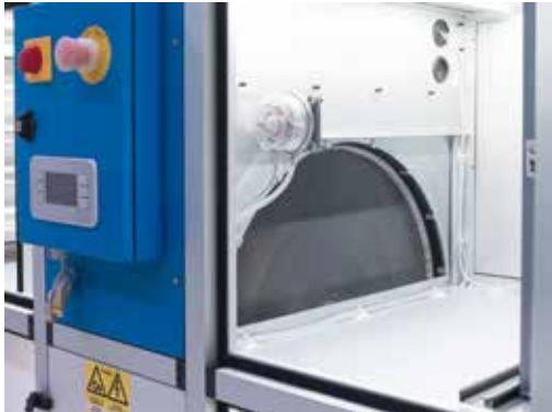
Heat wheel for heat recovery
